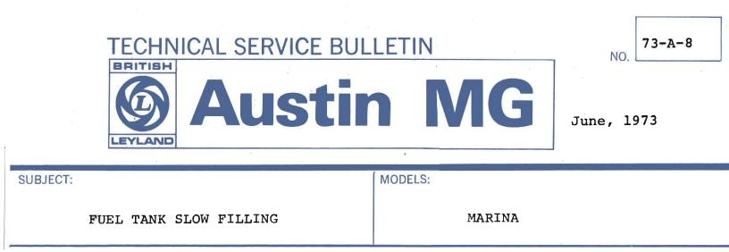
If this condition is encountered, it may be caused by a partially trapped or kinked breather tube.
