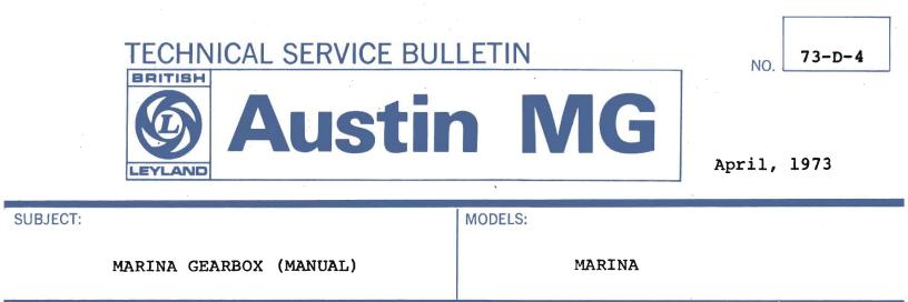
The drain plug has been deleted from the manual gearbox on the Austin Marina as it is considered unnecessary to replace the oil at servicing intervals. The gearbox will now require topping up only.
