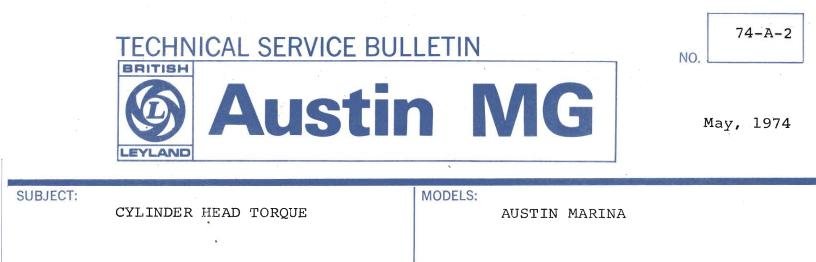
The cylinder head torque on the Marina has been increased from 45 - 50 lb./ft. to 50 - 55 lb./ft. Therefore, this information should be inserted in the appropriate section of your workshop manual.
