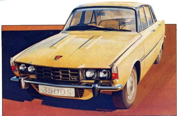
The light-alloy V8 engine was fitted into the P6 shell which had previously housed only the 2000cc and 2200cc engine to give the 120mph 3500 which found a ready executive market
