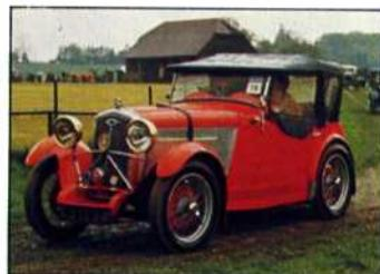
Above, the little Wolseley Hornet powered by a six-cylinder engine of only 1271cc
