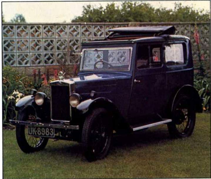
The original Morris Minor broke new ground for Morris Motors as it was the first overhead cam Morris and the first to have wire wheels, coil ignition and a dry-plate clutch as standard
