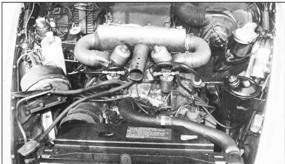
Above, the Buick-derived Rover V8 as fitted into the P6 giving the car performance and refinement never seen with the 2000 and 2200 models. The later 152bhp 3500S model, first introduced in 1971, had a four-speed manual gearbox replacing the three-speed automatic of the standard 3500
