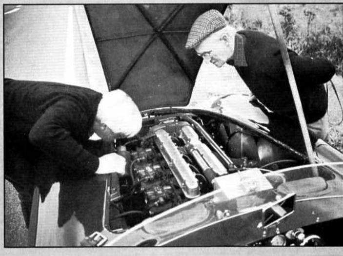
had to stop twice to let the engine cool down. Barry had fitted a Kenlowe to the normally fanless car, but stopping for more than a few seconds saw the temperature gauge rising inexorably. Switching off and keeping fingers crossed for a clean restart of the full-race engine was the only answer.
