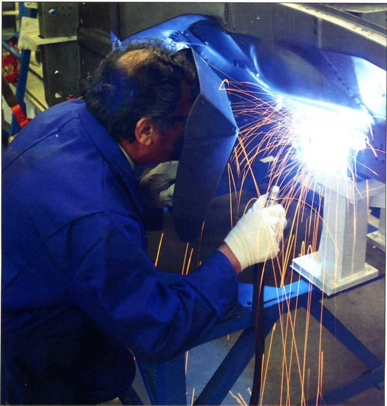
*Above, welding in progress on the new shell. Much of the original jiggging was adapted to carry out more than one task*
