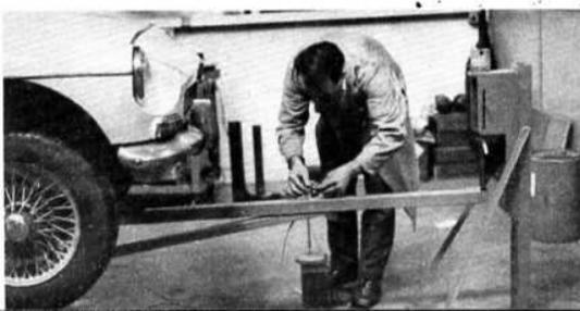
Setting up the MGC at Cranfield for pitch and yaw inertia measurements.
