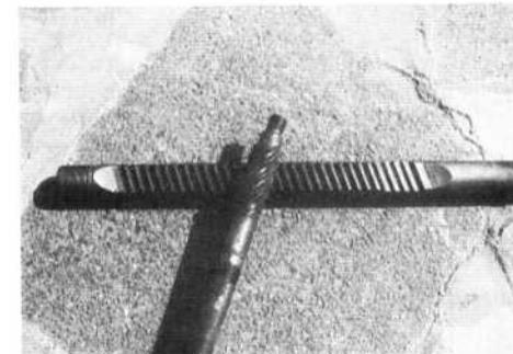
*Split steering arm gaiters let water in producing this badly pitted rack and pinion set.*
