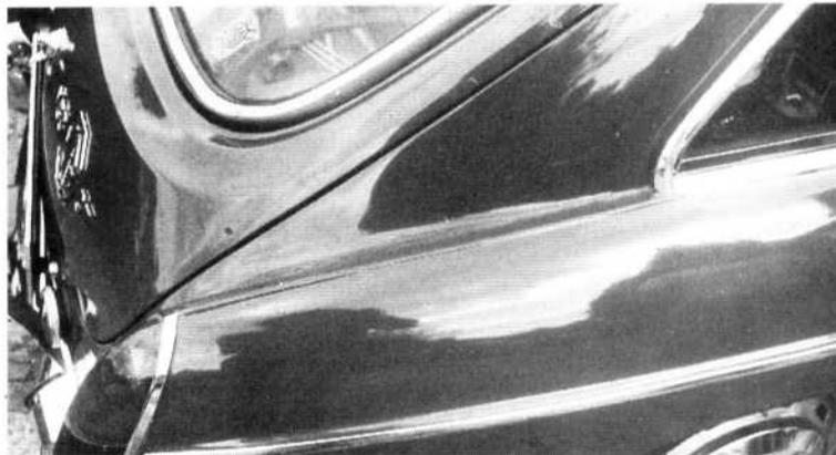
The bead on the rear wing top is a favourite area for rust bubbles. Below, boot space on the roadster is adequate but lacks trim.
